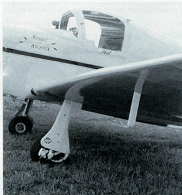
Manual operated landing gear contributes to the Cadet's great performance. Retractable gears were a rarity in the days when the Cadet was introduced—especially on an aircraft of this size.
